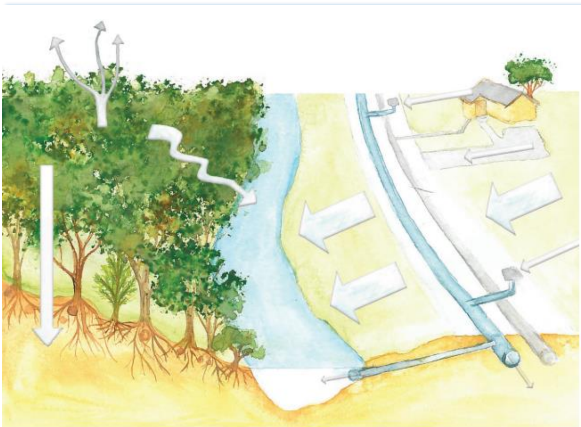
The water cycle. In natural landscapes, water slowly infiltrates into the earth, and runs off into rivers and streams (left). In urban landscapes, it quickly runs off impermeable surfaces (right).
